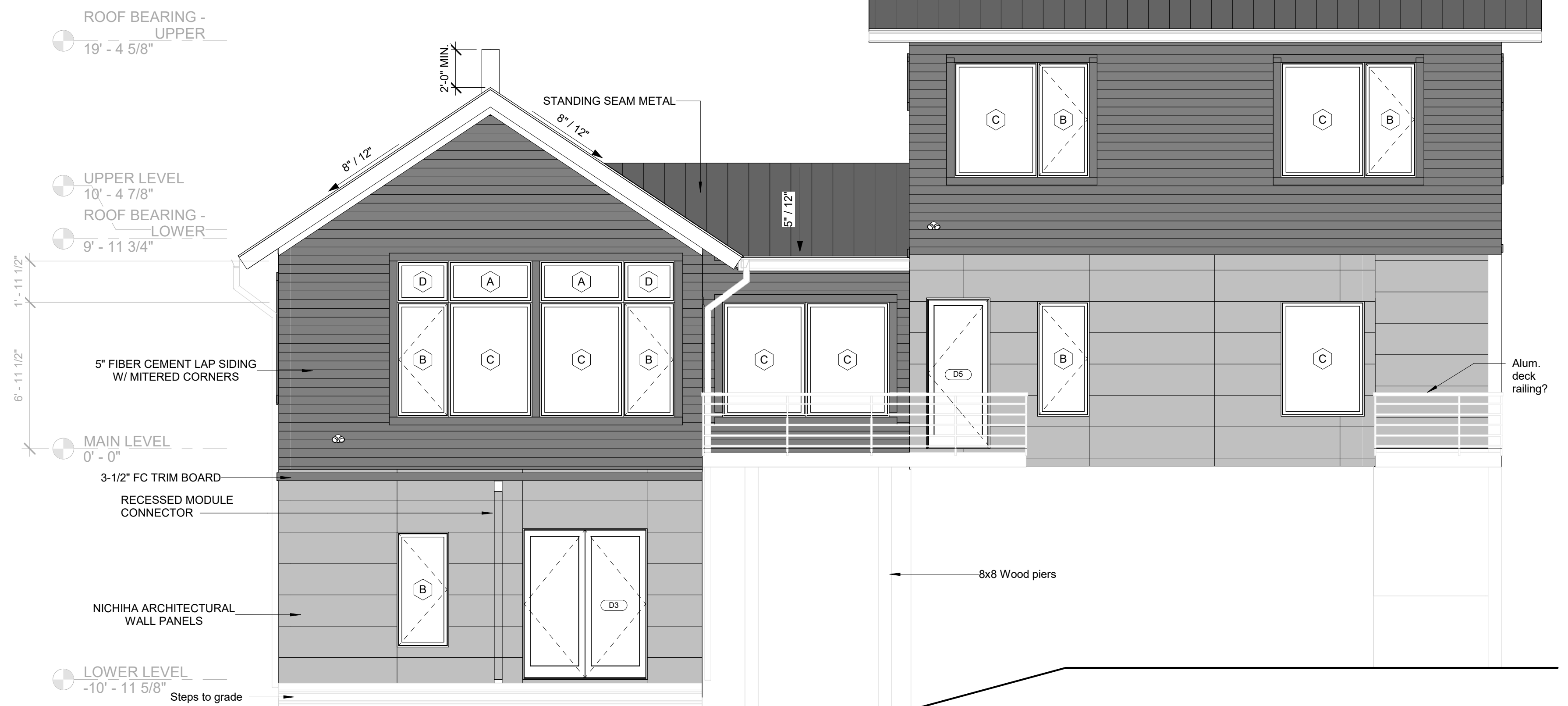
① Building Elevation - East 1/4" = 1'-0"
