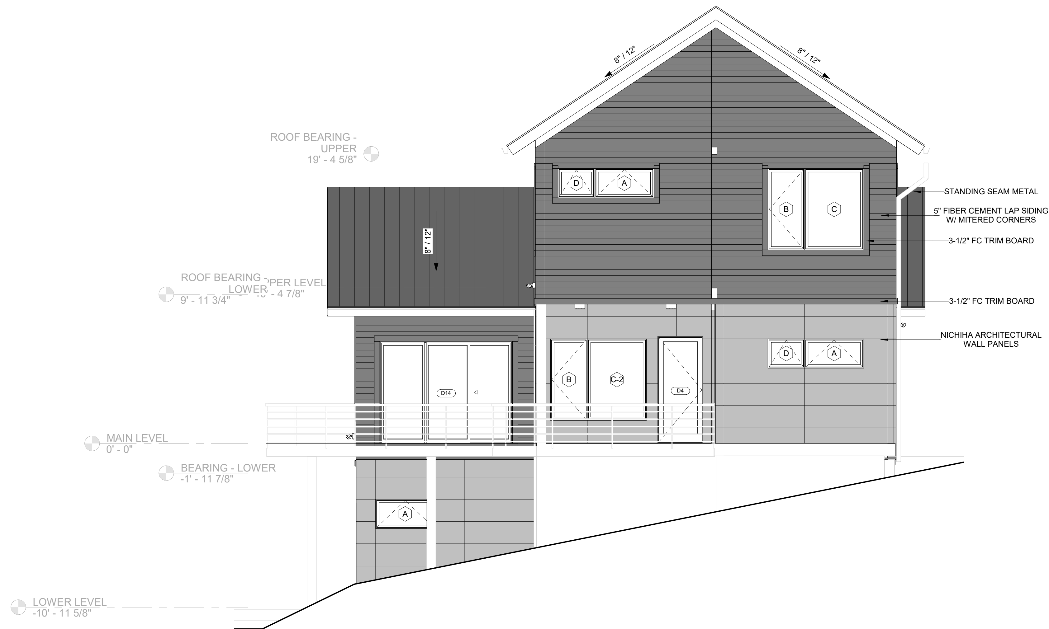
2 Building Elevation - North 1/4" = 1'-0"
